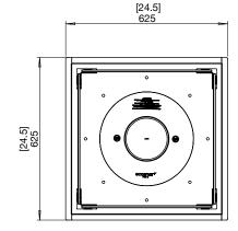
This model complies with existing standards in the USA, Europe, UK and Australia. O-TL listed to UL1370, EN 16647 BSI Certified and ACCC Safety Mandate compliant. \*\*To comply with EN 16647 the Indoor Safety Tray and included AB8 Burner Efficiency Ring must be installed before operating indoors.
